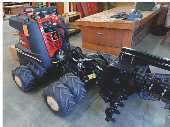
Dual wheels are optional. The trencher (and plow) is mounted to the InterChange connection via the low-lift tool carrier.
