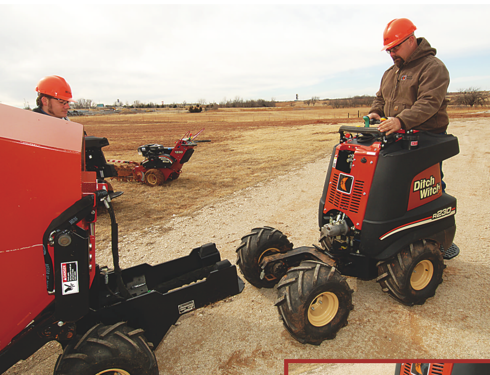
The Zahn's InterChange connection (right) engages the work tool (above), and the tool is secured via flip-up, threaded latches at the front of the InterChange frame.
