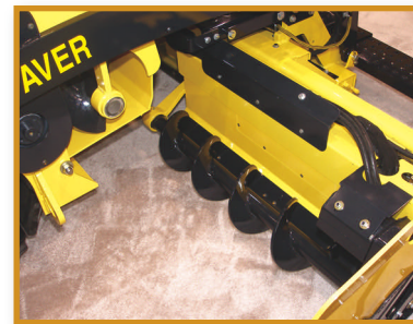
Top photo: Bomag's 20,500-pound 6615 is one of the first asphalt pavers by a traditional commercial-paver manufacturer that is heavier than the traditional 19,000-pound boundary defining the large end of the paver category. It employs Bomag's first electrically heated screed with bolt-on, 400-Brinell hardened steel screed plates and a Mega Feed system that includes augers mounted to the front of the extensions (inset).
