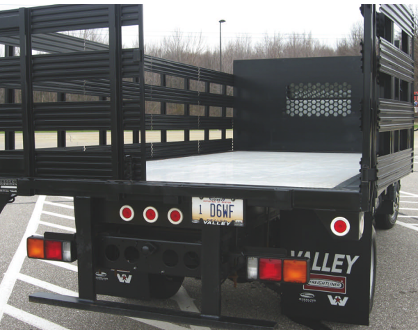
The 14-foot American stakebed body uses composite floor and sides.
