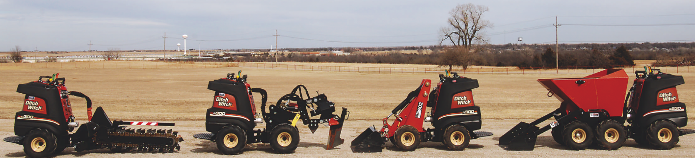
During CE 's visit, we used the Zahn in a number of configurations, including, from left, an R300 two-wheel-drive trencher, R300 vibratory plow, R300 high-lift tool carrier and an R230 dumper.
