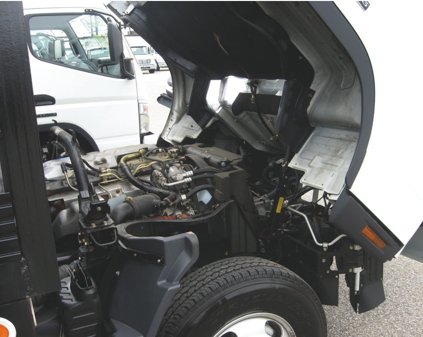
Above: Economical and adequately powerful inline 4-cylinder turbodiesel is readily accessible after the cab is tilted forward.
