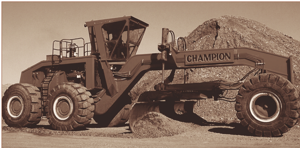
The 100T was a hydraulically operated grader with an articulated frame and tandem rear wheel drive. An 8-speed power-shift transmission provided a top speed of 35 mph.
