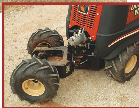
The Zahn's InterChange connection (right) engages the work tool (above), and the tool is secured via flip-up, threaded latches at the front of the InterChange frame.
