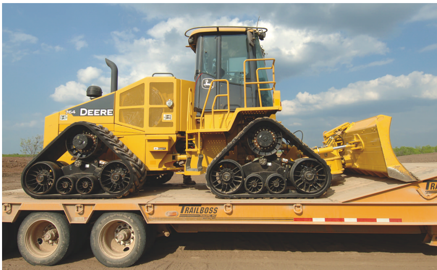
Mounting the cab on the tractor's front frame puts the operator close to the six-way dozer blade and looking straight down to the blade through the cab's broadest stretch of glass even in turns.
